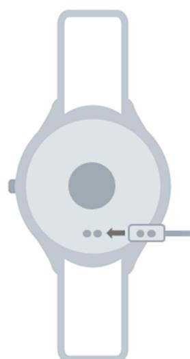
Before using your JOLI XW PRO for the first time, you should fully charge the battery of the JOLI XW PRO. Use the supplied charging cable.
